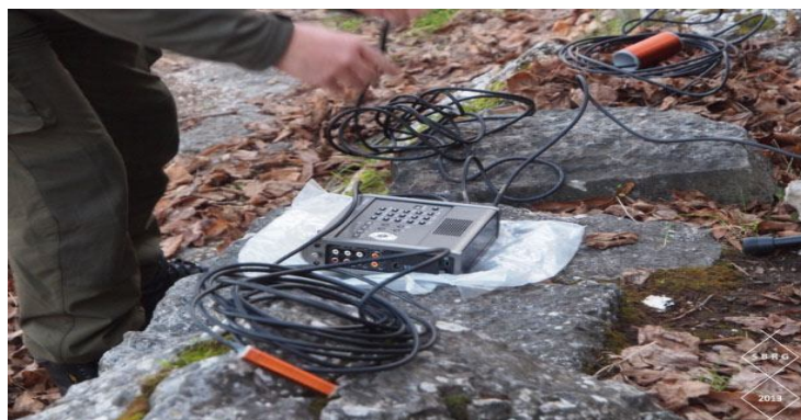
Fig. 7: The sensors with different sensitivity ( 300\Omega ) that transform electromagnetic impulses from the environment, into electrical impulses used by the digital recorder.
